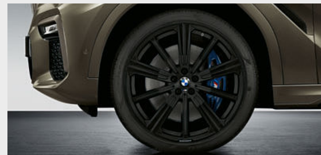
○ The high-quality 22" M Performance light alloy wheels Star-spoke style 749 M are weight-optimised with flow forming and designed in Jet Black matt with the M Performance lettering and the colour M logo. TPMS summer complete wheel set, wheel size 9.5J x 22 with tyre size 275/35 R22 104Y XL at the front and 10.5J x 22 with 315/30 R22 107Y XL at the rear.
